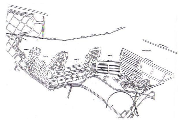
The **Port of Beirut Rehabilitation and Extension project** consist of **4 docks, 2 new quays (15,16) and a new container terminal** with 700,000 TEU/year capacity.
